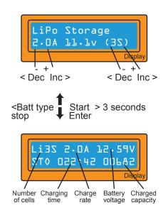
Here you can input the current and the voltage of the battery pack to be charged. The current will be used to either charge or discharge the battery in order for it to reach the ideal 'STORAGE' level voltage.
