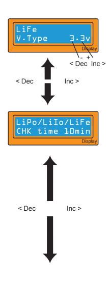
The screen displays the nominal voltage of the Lithium battery. There are four kinds of Lithium battery; LiFe (3.3V), Lilon (3.6V), LiPo (3.7V) or LiHV (3.8V). It is very important that you check the battery carefully to ensure it is set up correctly. If the incorrect values are selected the battery could ignite or explode during the charging process.
