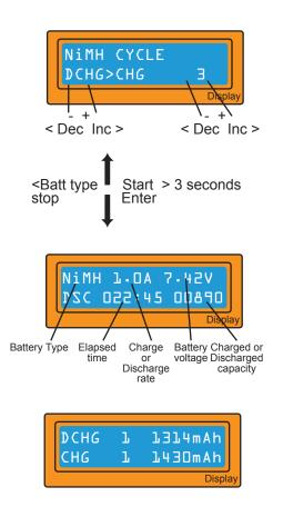
On this screen you can alter the cycle sequence on the left and the number of cycles on the right. The 'CYCLE' mode can be used for balancing, refreshing and 'breaking-in' the battery. A time delay will occur after each charge and discharge process to allow the battery adequate time to cool down before being subjected to the next process. This delay is set on the 'User Settings' menu.
