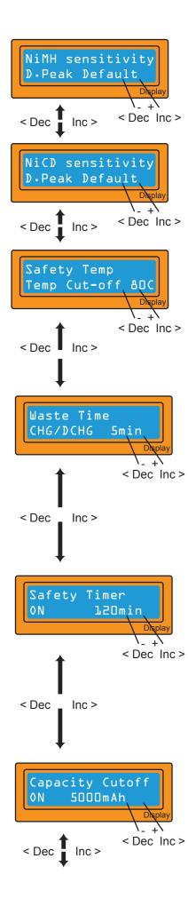
This shows the trigger voltage for automatic charge termination of NiMH and NiCd battery. The effective value ranges from 5 to 20mV per cell. If the trigger voltage is set higher, there is a danger of overcharging the battery; if it is set lower, there is a possibility of premature termination. Please refer to the technical specifications of the battery. (NiCd default: 12mV, NiMH default: 7mV)
