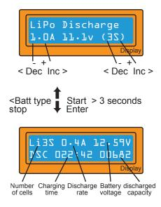
The discharge current (shown on the left side of the screen) should not exceed 1C and the final voltage on the right should not be under the voltage level that is recommended by the battery manufacturer to avoid deep discharging. To start the discharge process, hold **Start/ Enter** key for 3 seconds.
