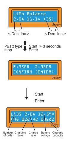
On this screen the first value on the second line is the charge current and the second value is the voltage of the battery pack.
