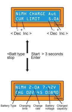
This program charges the battery using the charge current set by the user. In 'Aut' mode, you must set the charge current limit to prevent the charger feeding too much current into the battery, which could cause damage. In 'Man' mode, the battery will be charged with the charge current set by the user. You can change the mode by pressing **INC** and **DEC** button simultaneously when the current field is blinking.
