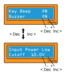
The beep sounds every time a button is pressed to confirm your action. Beeps or melodies may be sounded at various times during operation to alert the user of different mode changes. You can turn these sounds on and off.
