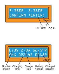
This shows the number of cells within the battery pack. 'R:' is the number of cells found by the charger, and 'S:' is the number of cells selected by the user on the previous screen. If both numbers are identical you can start charging by press **Start/Enter**. If not, press **Batt Type/Stop** to go back to previous screen to modify any incorrect information that may have been input by the user.
