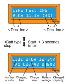
You can set up the charging current and the voltage of the battery pack which is being charged. Press **Start/Enter** to bring up the voltage confirmation screen. If the voltage and current parameters are correct, press **Start/Enter** again to start the charging process.
