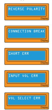
The output is connected to a battery with incorrect polarity.
