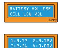
This screen will appear if the processor finds that the voltage of one of the cells in the Lithium battery pack is too low.
