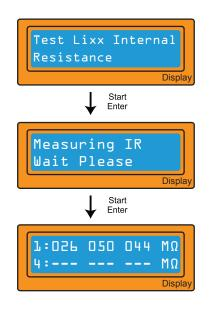
Select the interface for Internal Resistance Testing. Press **Start/Enter** to enter into it.
